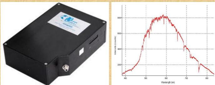
The HR4000 high-resolution spectrometer with a 3648-element CCD-array enables optical resolution as precise as 0.02 nm (FWHM). The specific range and resolution depends on the grating and entrance slit choices.
