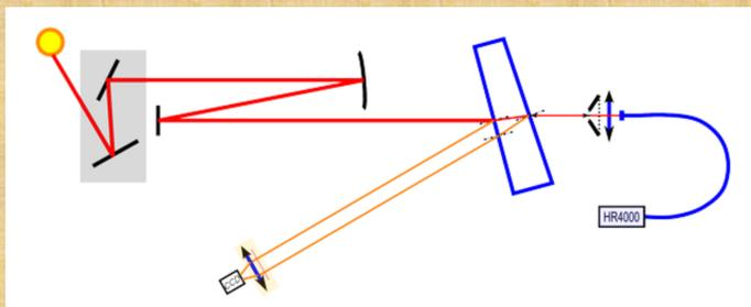
Horizontal solar telescope HSFA2 (red line) creates solar disk image  $\Phi$  32 cm at the optical surface (blue wedge). Light is partly reflected to the H $\alpha$  telescope (light brown) and partly enters to the light collector through one of 7 diaphragms placed on a rotating wheel. Optical cable (blue arc) feeds the spectrometer HR4000 (right down).
